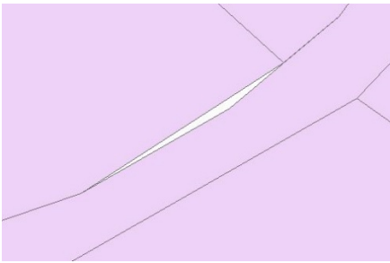
Gap that needs removal
